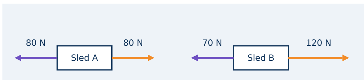
Horizontal forces on sled A and sled B.
