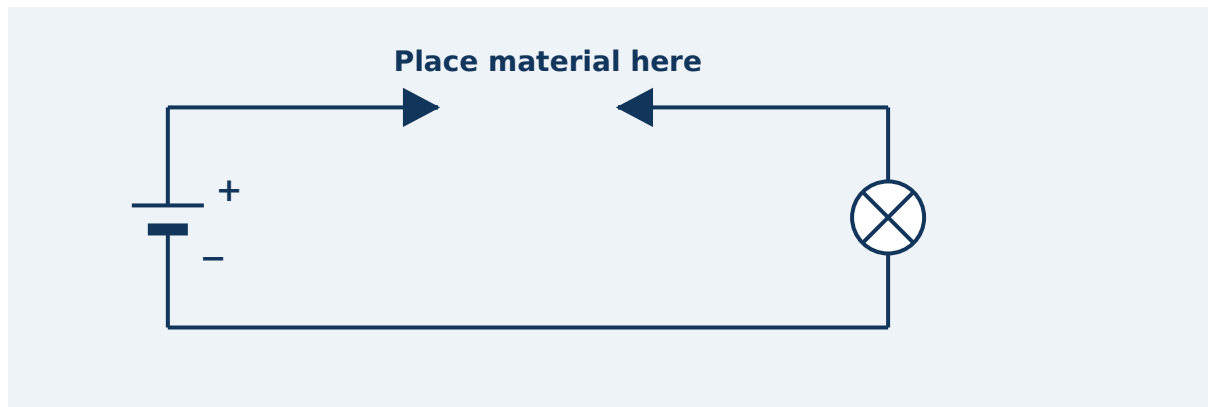
A tester circuit used to find out whether a material conducts.
